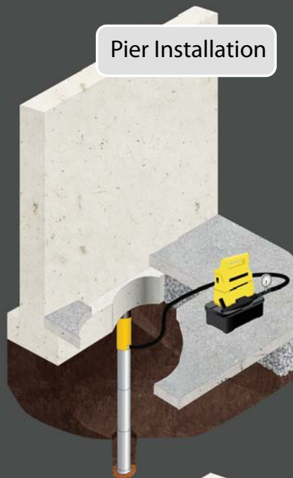
Footing Excavation & Preparation
