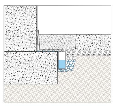
System components are manufactured from a high-strength thermoplastic compound. The system consists of extruded rectangular drainage channels, couplings, 90° & 45° corners, drain outlets and clean outs. Lineal sections are manufactured as hollow rectangular tubes having slots in the exterior vertical face to allow the entrance of ground water. Water travels through the system to outlet fittings which provide the connection of ECP SDS to our ECP Sump Basin.
